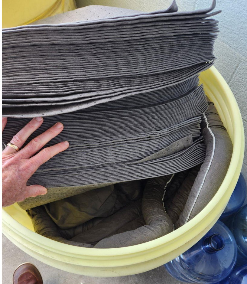
Figure 1 - Typical Drum Spill Kit located on each Island at the Ventilation Building and Maintenance Yard.
